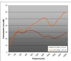
OL 12-0201 – Reference wall before application of Green Glue Noiseproofing Sealant – STC 24
