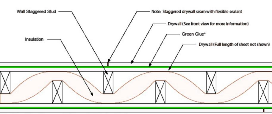
Note: \*Green Glue will have no real thickness in finished construction
