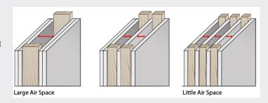
To make matters worse, each leaf in the double leaf wall is very heavy, but each leaf in the quadruple leaf wall is far lighter – half the mass. This will cause resonance to go up in frequency even more, and low frequency performance will be badly degraded.
